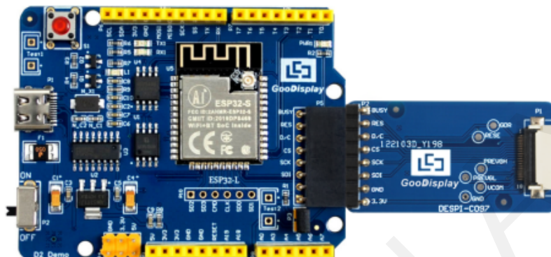
Figure 3 : Connection between ESP32-L for EPD and DESPI-C097
